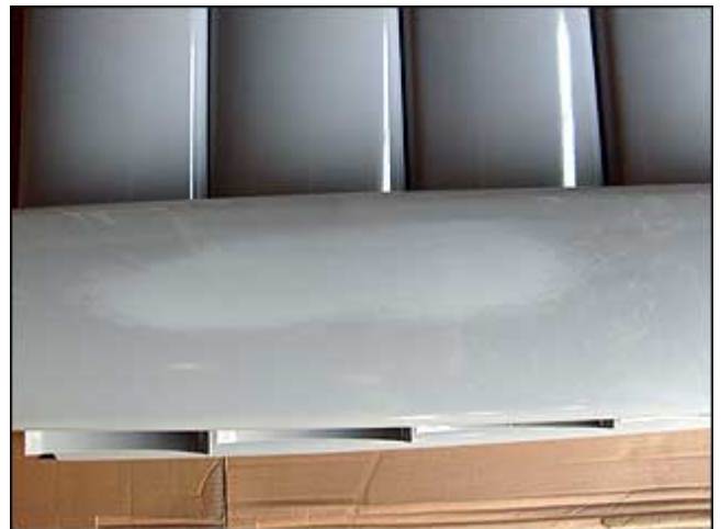
Example of sanded piece which must be reworked.
