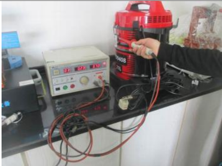
High voltage test
