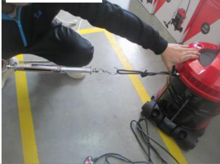
Power cord strain relief test
