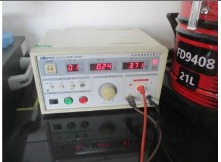
High voltage test
