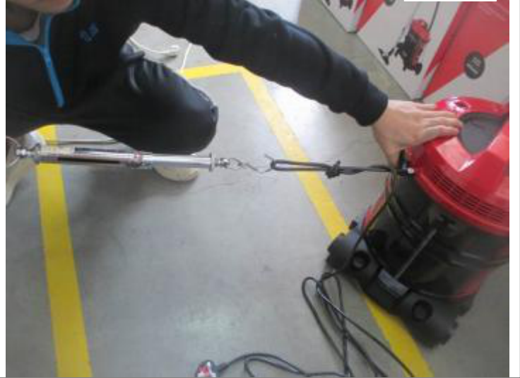
Power cord strain relief test
