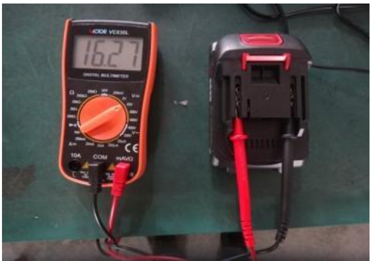
Battery voltage after discharge
