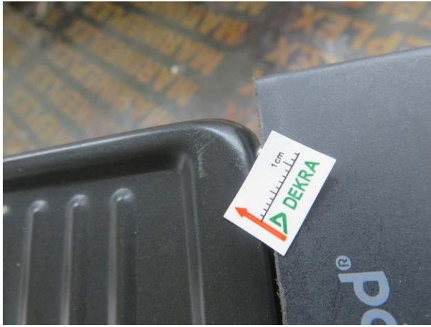
97) Minor - Scratch mark on heating plate
