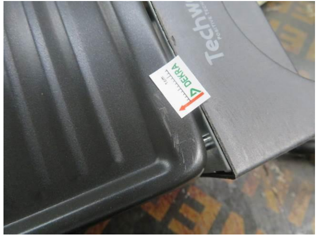
98) Minor - Scratch mark on heating plate
