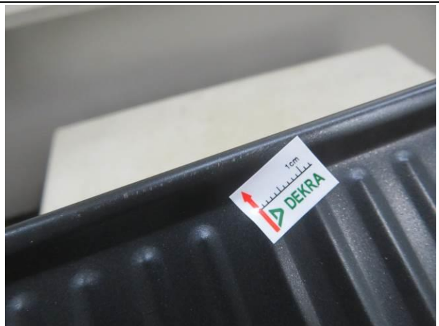
96) Minor - Scratch mark on heating plate
