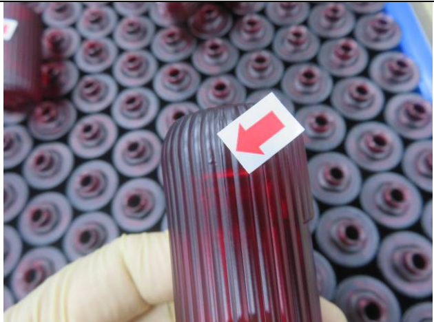
Poor sanding –Minor
