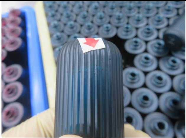
Poor sanding –Minor
