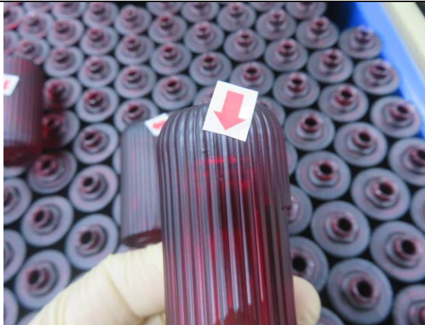
Poor sanding –Minor
