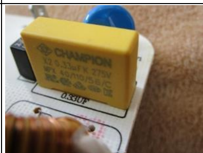
X2 capacitor: MPX 0.33uF 275VAC Champion
