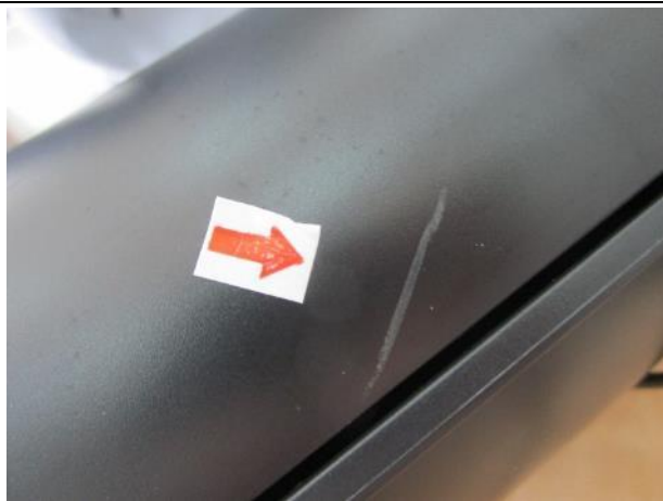
Scratch mark on housing ---4pcs Minor
