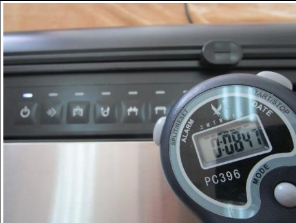
Sealing time of dry pumping- 8-10S
