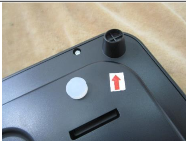
One silicone foot loose out ---3pcs Major
