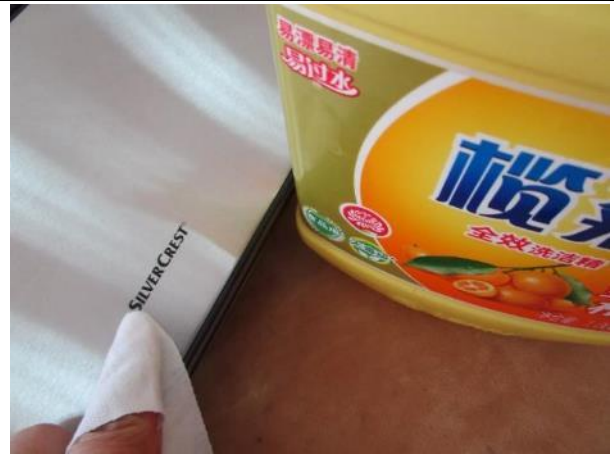
Rubbing test with washing-up liquid
