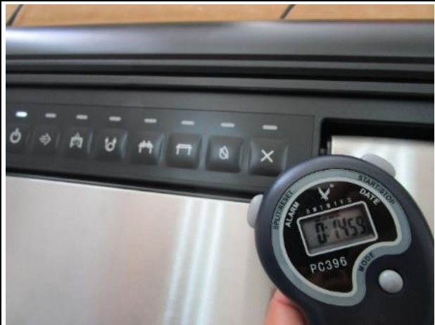
Sealing time of wet pumping-12-14S
