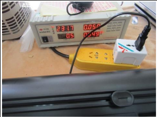
Standby power check
