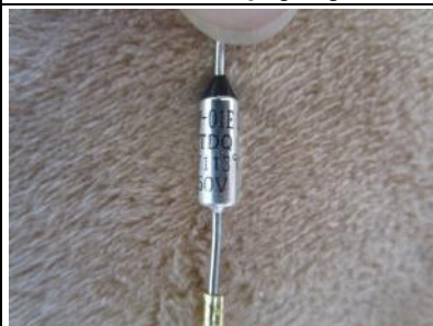
Thermal link: RY-01E113 10A 250V, Tf113°C
