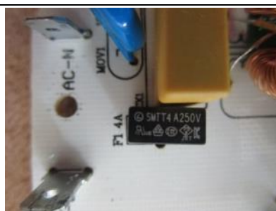
Current fuse: SMT T4A 250V
