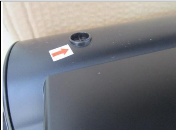
One silicone foot loose out ---3pcs Major
