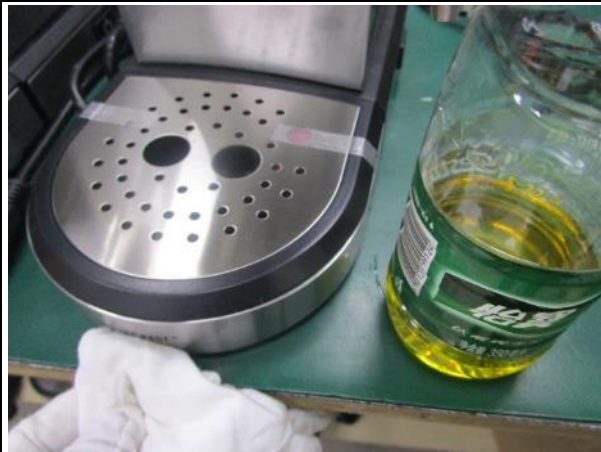
Rubbing test with vegetable oil
