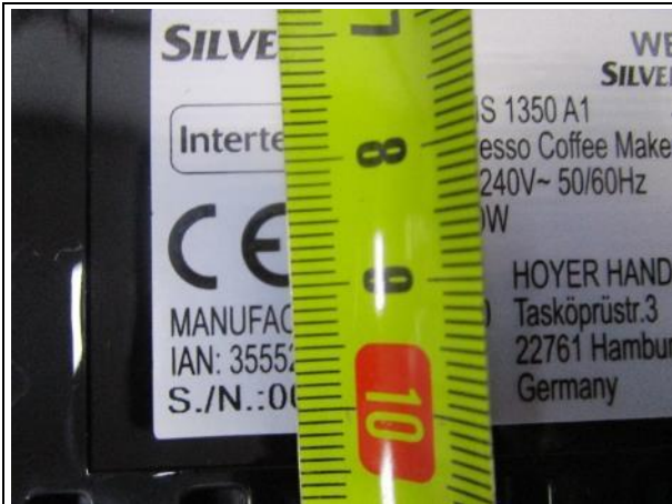
CE mark height: min 5mm
