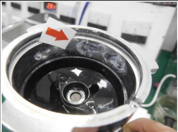
Step between upper and lower body---3pcs Minor
