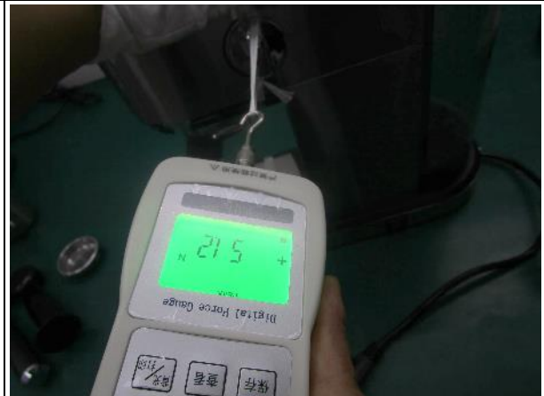
Pull test for knob: 50N
