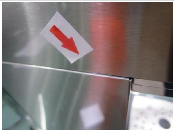
Step between upper and lower body---3pcs Minor
