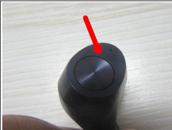
The knob is lower than the surface of the housing - 5pcs
