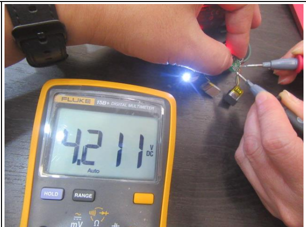
Battery voltage of full charged
