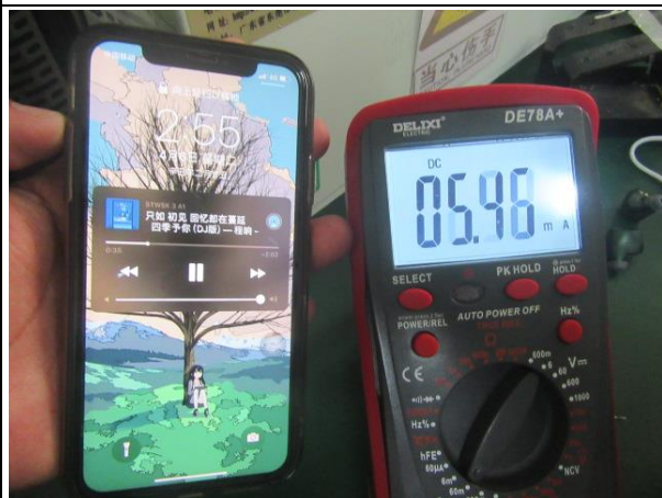
Working current test
