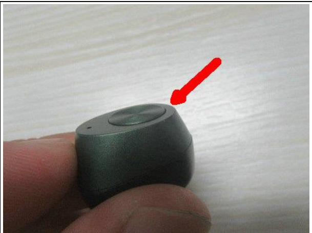
The knob is higher than the surface of the housing - 3pcs
