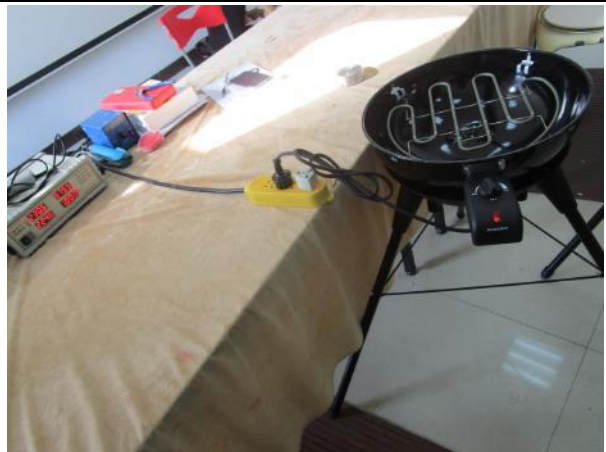
Input power test
