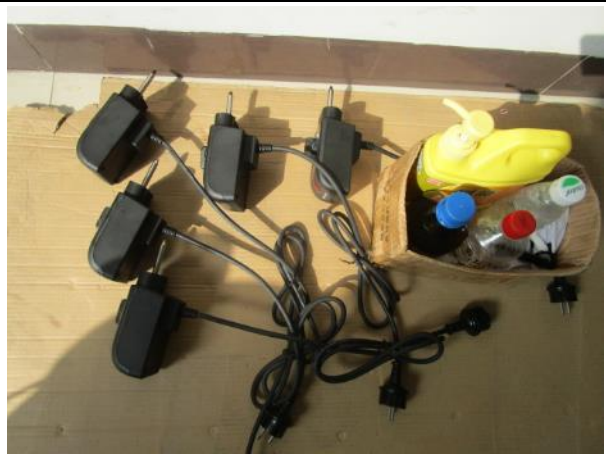
Rubbing test after 12h with vegetable oil (6h only)
