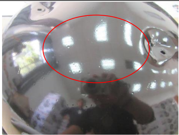
Poor coating of the base housing-2pcs Min
