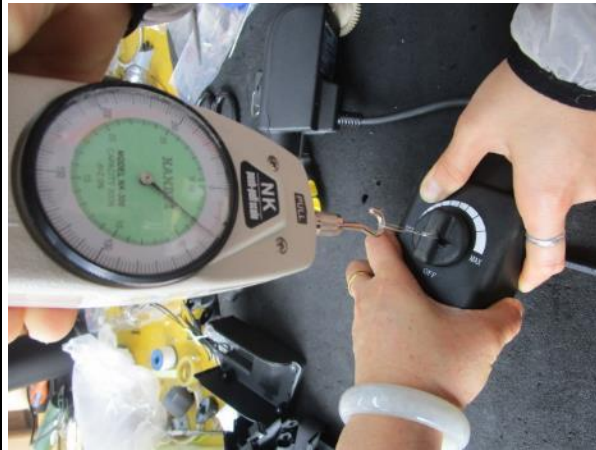
Control knob pull test:30N
