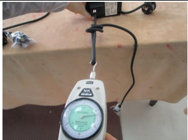
Power cord pull test: 60N
