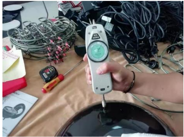
Enamel coating impact test
