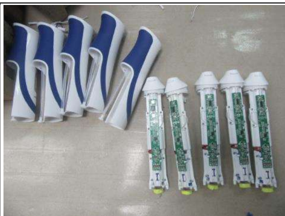
Internal check after 10 mins water proof test
