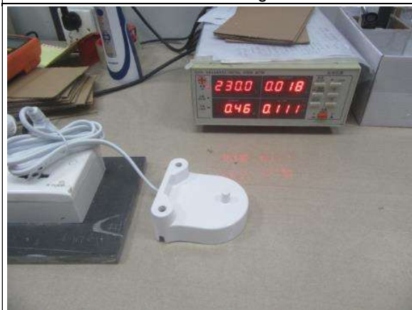
Charger base standby power (<0.5W)
