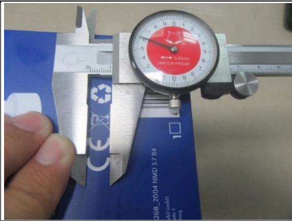
CE mark height: min 5mm
