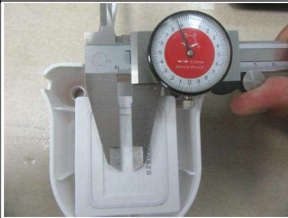
CE mark height: min 5mm
